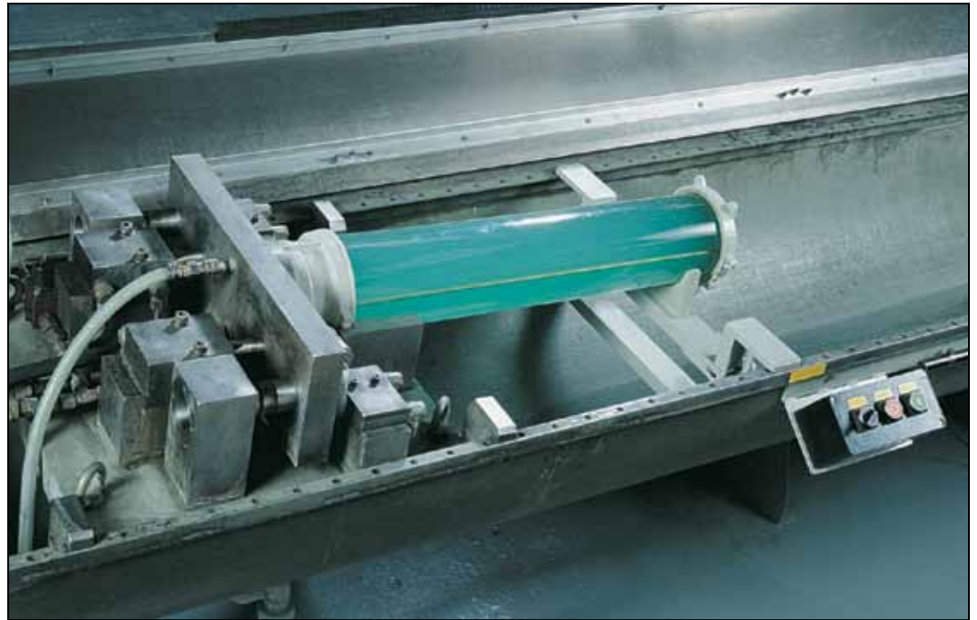
RIGOROUS CHECKS ARE PERFORMED AT EACH STAGE OF THE MANUFACTURE OF ATX EQUIPMENT. HERE, AN INDIVIDUAL OVER-PRESSURE TEST ON A FLAMEPROOF « d » ENCLOSURE IS BEING PERFORMED ON THE PRODUCTION LINE.
