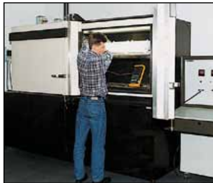
CLIMATIC TESTS -50 °C UP TO + 200 °C. WITH 0 UP TO 100 % OF RELATIVE HUMIDITY.
